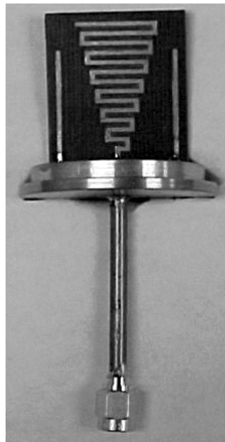
FIGURE 12.44 The prototype of dual-sleeve taper meander line with e_1 = 2 mm and e_2 starting from 3 mm and ending with 17 mm on a 29-mm dielectric slab. (From ACES J. , 15(3), 159, 2000.)
