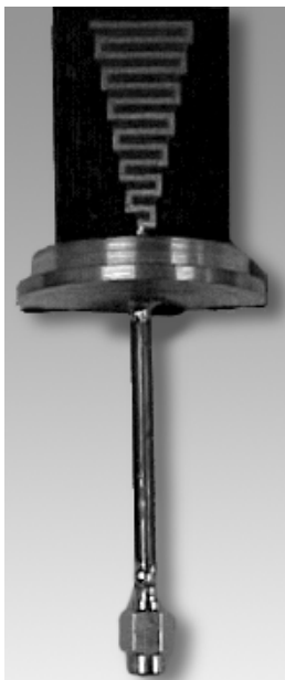
FIGURE 12.43 The prototype of taper meander line with e_1 = 2 mm and e_2 starting from 3 mm and ending with 17 mm on a 29-mm dielectric slab. (From ACES J. , 15(3), 159, 2000.)
